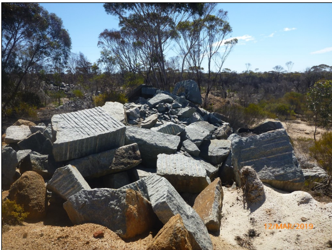
Plate 11: One of many reject block stockpiles
